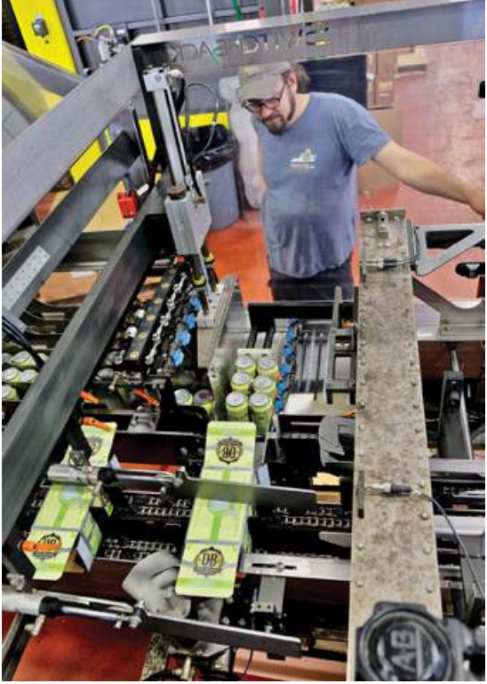
Cans are packed into cartons on a Brewpack 150.
