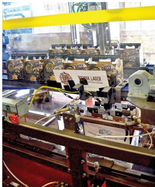
Paperboard basket-style carriers are erected and stuffed into cases that then are fed into the drop packer.
