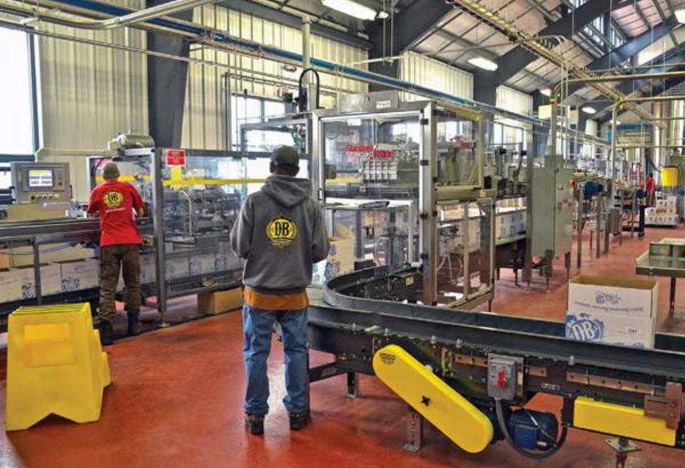
Operators attend to the case erector and drop packer on the Devils Backbone bottling line.
