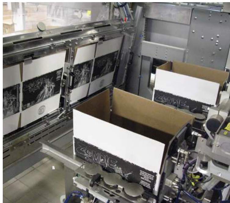
Vacuum cups pick two cases at a time from a magazine feed and erect them so that they can be positioned for folding and gluing of their bottom flaps.
