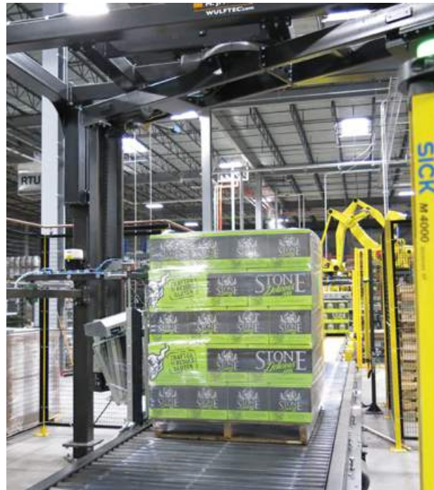
Palletized cases are stretch wrapped before coming off the line.
